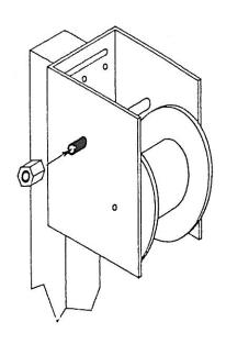
(B.) ATTACH DRIVE SHAFT GUIDE TO UPRIGHT USING EXISTING WINCH EDLTS.
