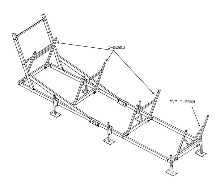
(A) ATTACH THE (2) 20' TOP RACK BEAMS TO THE TOP OF THE I-BEAMS USING 1/2" X 3 1/2" MACHINE BOLTS & 1/2" LOCK NUTS. DO NOT OVERTIGHTEN THE LOCK NUTS BECAUSE THE TOP RACKS NEED TO BE ABLE TO MOVE FREELY!!
