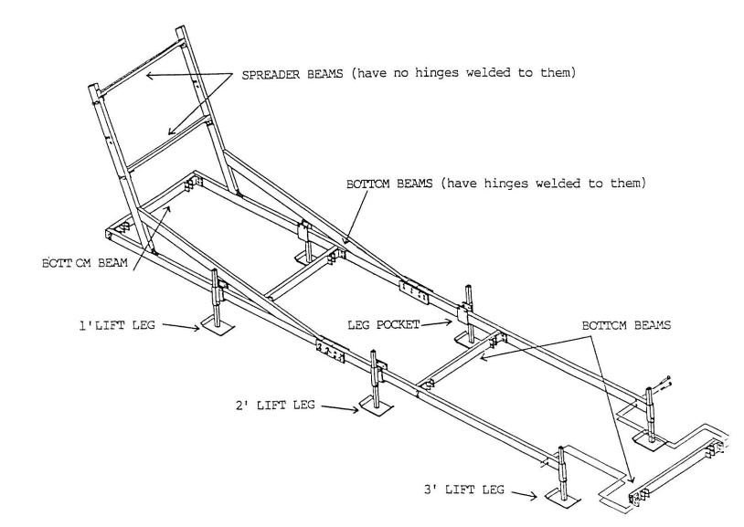
(A) BOLT THE I-BEAMS TO THE HINGES ON THE BOTTOM BEAMS AS SHOWN IN THE PICTURE USING 1/2" X 3 1/2" MACHINE BOLTS & 1/2" LOCK NUTS. DO NOT OVERTIGHTEN THE LOCK NUTS BECAUSE THE I-BEAMS NEED TO BE ABLE TO MOVE FREELY!!!
