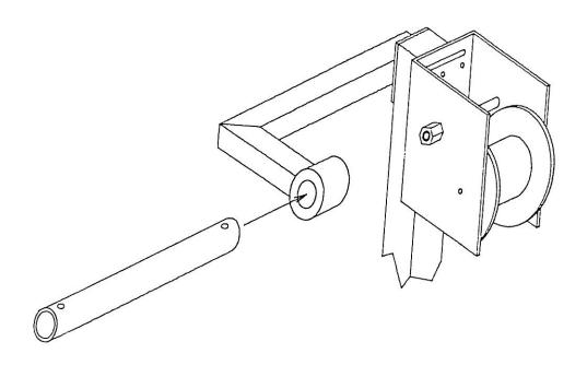
(E.) THEN SLIDE THE LIFT WHEEL INTO THE 2' WINCH DRIVESHAFT EXTENSION AND SECURE IN PLACE USING SET SCREWS.
